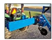
Optional 72-inch and 84-inch sliding offset mounts give you the flexibility to get you close and tackle a variety of work conditions. Handy storage slots keep parking stands securely contained during operation.
