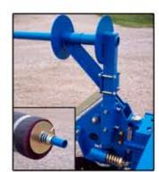
Height-adjustable roll holder allows for a variety of fabric roll lengths.
