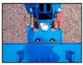
Forward pivot provides a 40° swing to either side of center. Couple this with an offset mount, and you get a supertight turning radius
