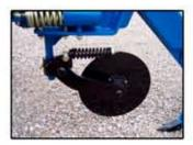
Spring-loaded, hardened-steel coulter with its unique curved arm cuts through trash, roots, and virtually any soil type.
